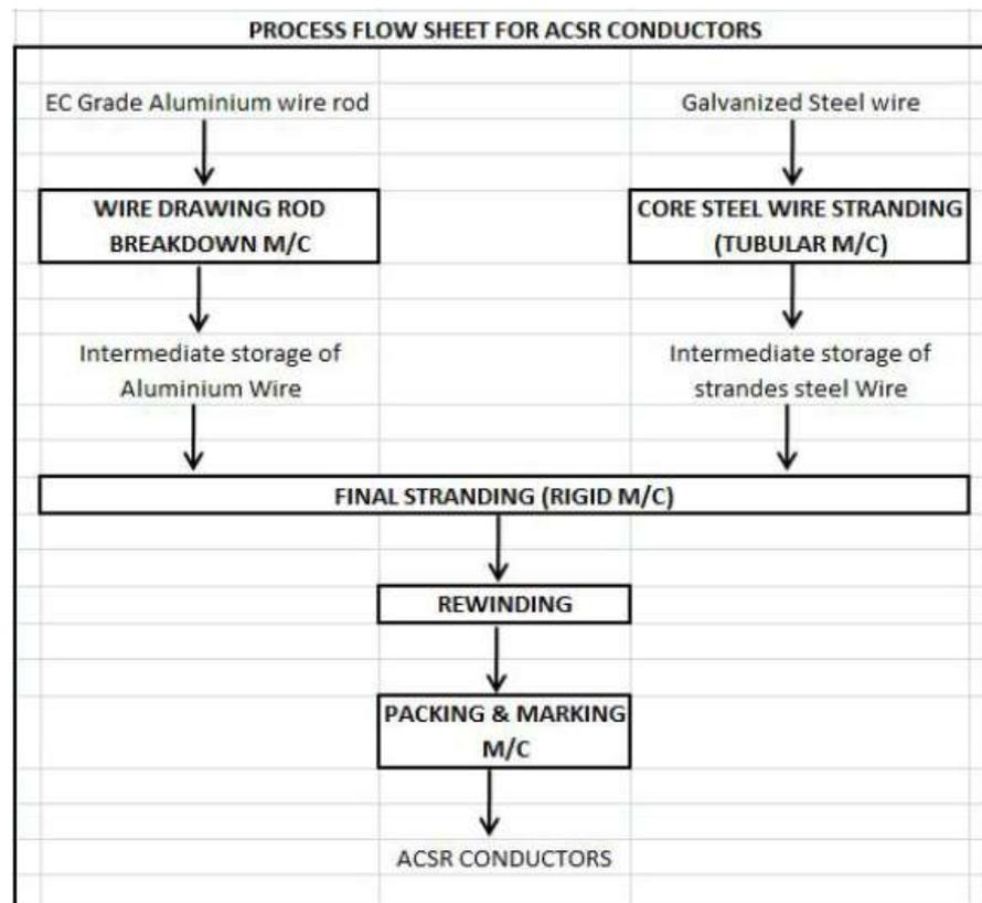
During the aluminium wire drawing, the multi-stage reduction of aluminium wire rod is carried out through passage of successive dies of decreasing die aperture by means of a tensile force applied at the exit side of each die. The aluminium wire are loaded in the skip stranding machine for aluminium core stranding.
