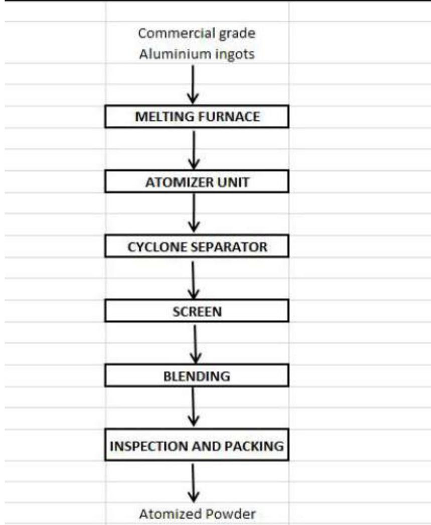
Testing of the products is followed by the last step of the process, viz. packaging, which ensures product safety from any outer mechanical damage as well as protection from moisture and contaminants.
