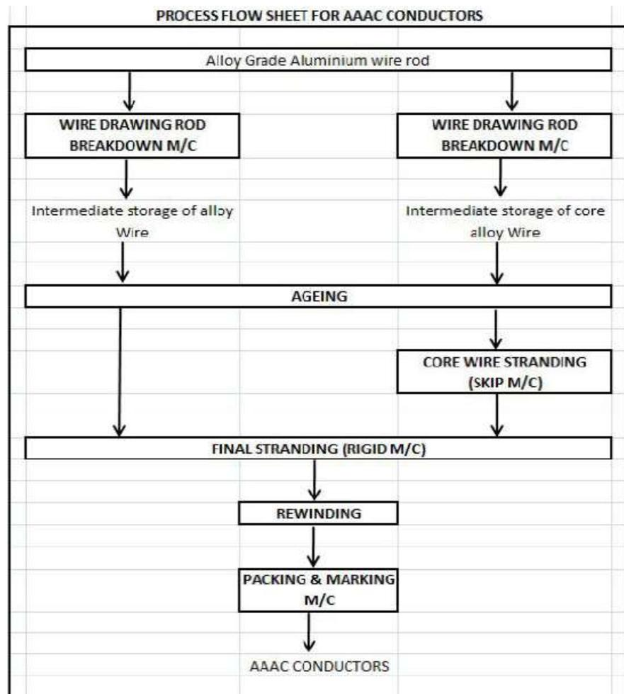
During the aluminium wire drawing, the multi-stage reduction of aluminium wire rod is carried out through passage of successive dies of decreasing die aperture by means of a tensile force applied at the exit side of each die. The aluminium wire are loaded in the skip stranding machine for aluminium core stranding.
